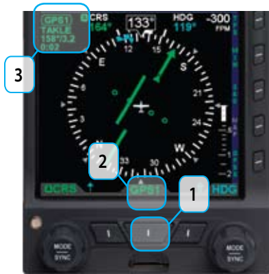
Figure 4-56 Navigation Source Information Block
