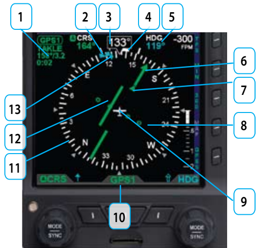
Figure 4-32 Horizontal Situation Indicator
